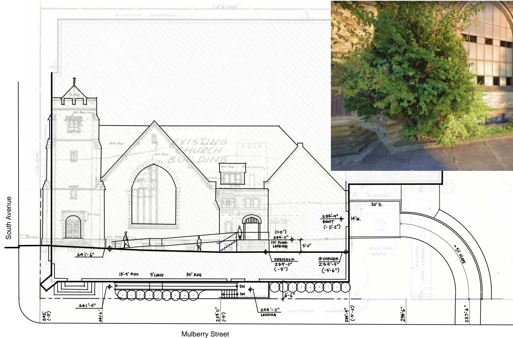
Ramp Plan and Elevation Scale 1" = 20'-0" * Updated survey needed to verify fitout
